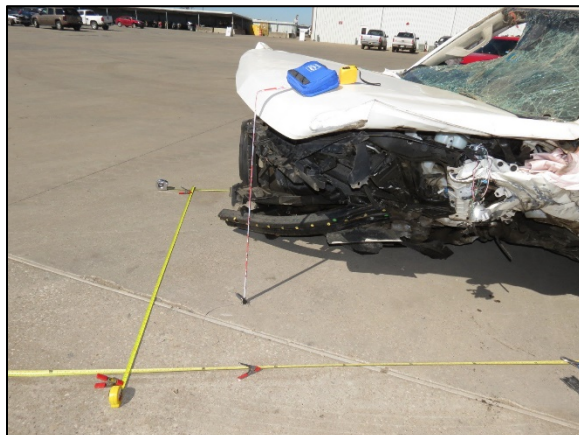
Figure 7: Crush to Chevrolet's bumper bar and hood
