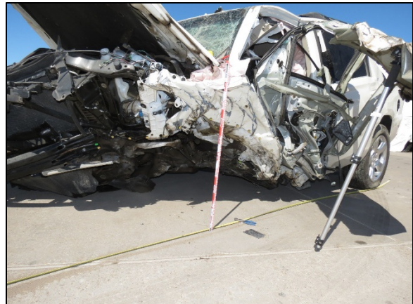
Figure 8: Damage to the undercarriage, fender, sill and left front door of the Chevrolet
