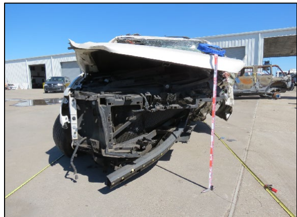
Figure 5: Damage to the front plane from the impact with the bridge support pillar
