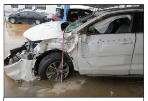
**Figure 3**. Damage from impact with end terminal.
