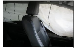
**Figure 7**. Left IC air bag impeded by left seat back and intruded B-pillar.
