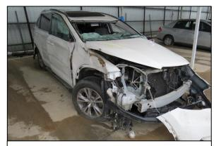
Figure 6. Right side rollover damage.
