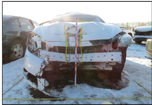
Figure 4: Damage to front plane of the Chevrolet from end terminal impact
