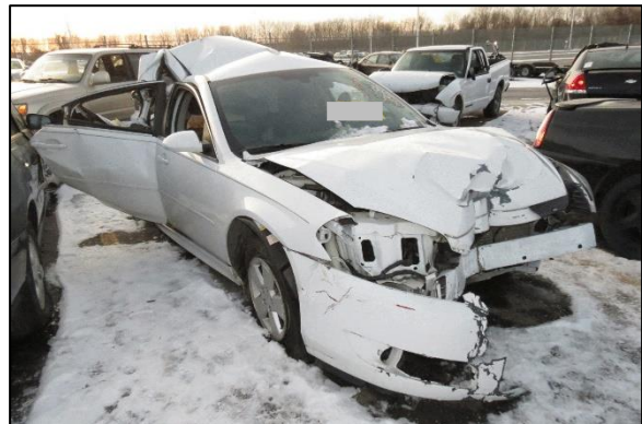
Figure 2: The damaged 2011 Chevrolet Impala
