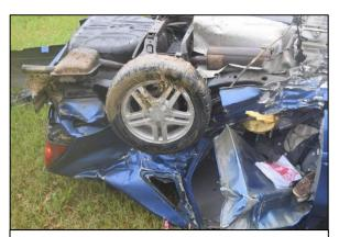
**Figure 6**. Police on-scene photo showing damage to the Ford's left rear wheel and quarter panel from ET-2000 impact.
