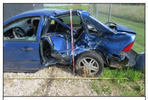
**Figure 4**. Left plane damage to the Ford from impact with the ET-2000.
