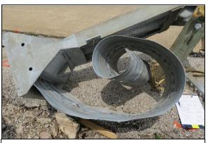
**Figure 9**. Guardrail extruded to field side from end terminal.
