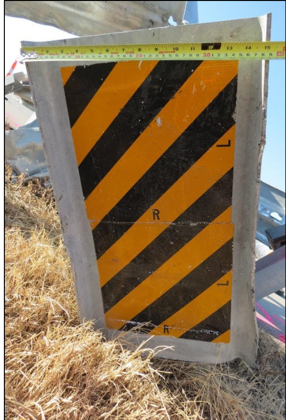
Figure 5. The face of damaged ET-Plus.
