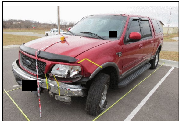
Figure 2. The damaged 2002 Ford F-150.
