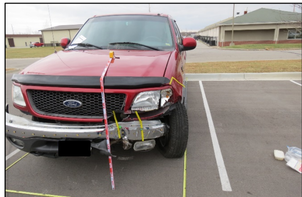
Figure 7. Damage from guardrail impact.
