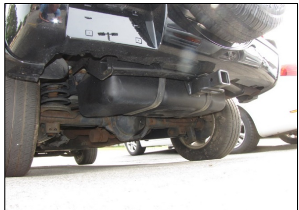
Figure 15. Rear view of the fuel tank and its location on an exemplar Jeep Liberty.
