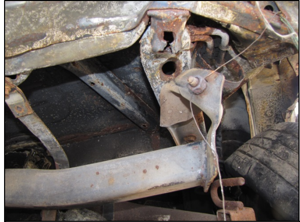
Figure 9. Forward-looking view of the right aspect of the Jeep's trailer hitch and the deformed right frame attachment bracket.
