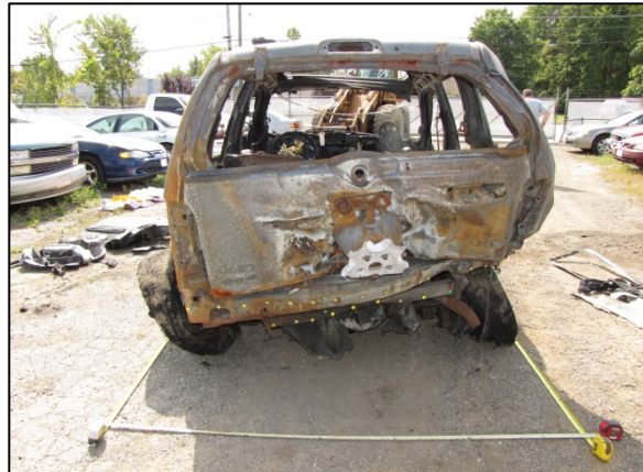
Figure 1. Back view of the Jeep Liberty depicting its deformation and fire damage.
