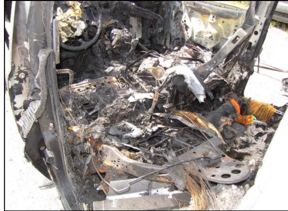
Figure 13. Interior view of the Jeep at the second row left looking forward.
