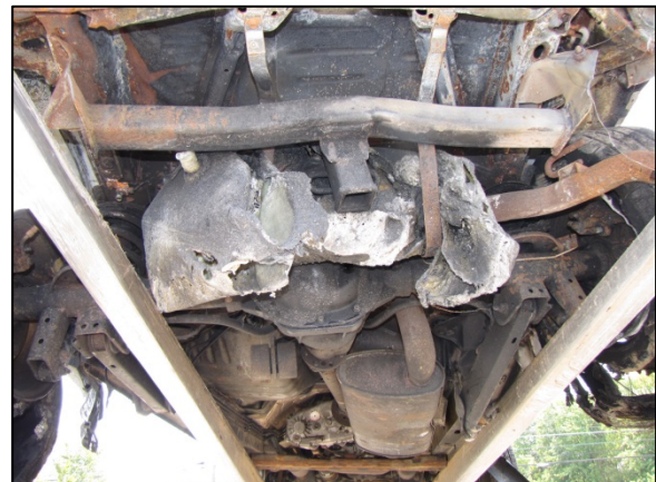
Figure 17. Undercarriage view of the Jeep's deformed trailer hitch and melted fuel tank.
