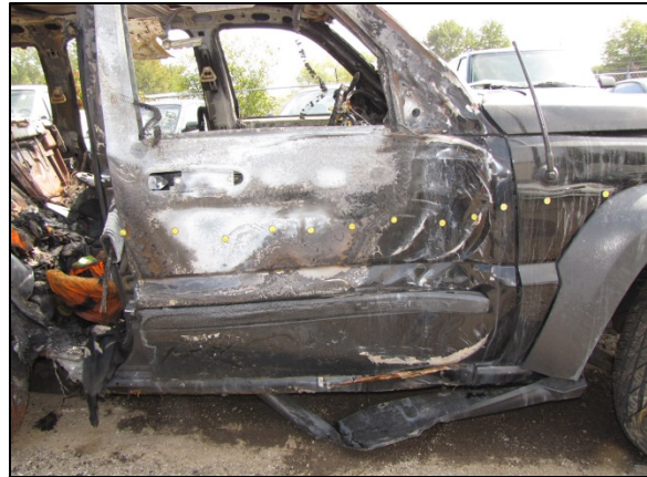
Figure 12. Right view depicting the Jeep's pole impact damage.
