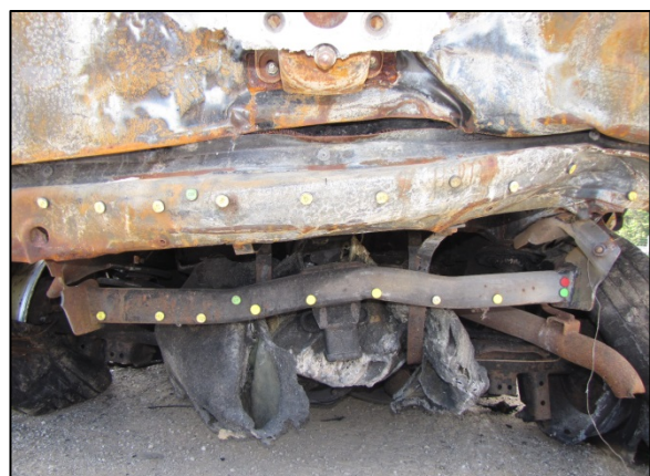
Figure 8. Forward-looking view of the Jeep's deformed trailer hitch.
