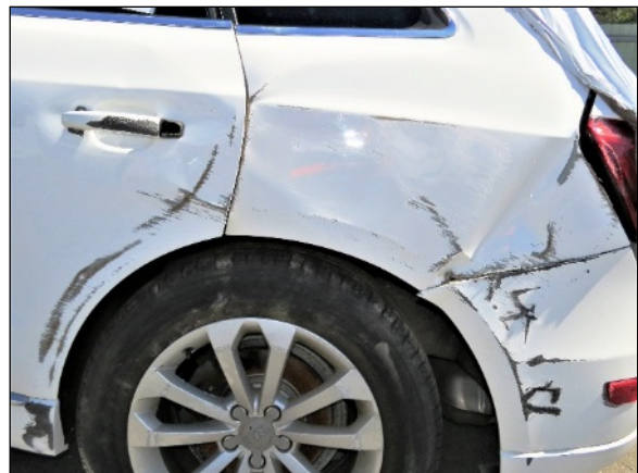
Figure 10. Close-up view of the diagonally oriented abrasions to the rear left aspect of the Audi.
