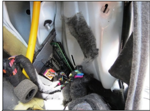
Figure 16. Crushed electronic module located in the right rear quarter panel area of the Audi and directly involved in the Event 1 impact deformation.
