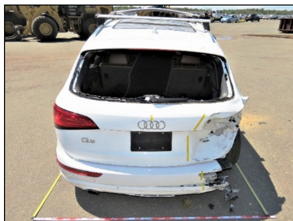
Figure 8. Back-plane view of the Audi’s damage profile as documented during the SCI vehicle inspection.
