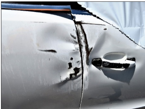
Figure 9. Close-up of the vertically oriented abrasions to the right doors of the Audi from the rollover.
