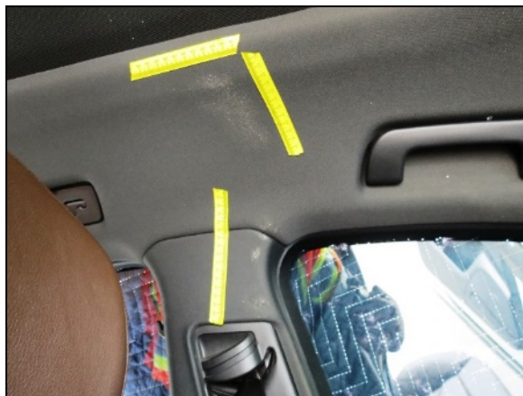
Figure 11. Skin transfer from the driver's head on the left roof side rail and upper left B-pillar.
