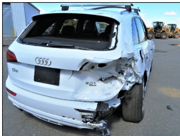
Figure 7. View of the Audi’s Event 1 damage pattern from impact by the Acura.
