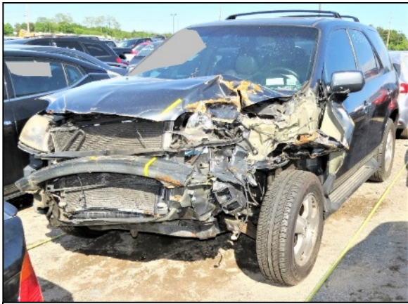
Figure 18. View of the Acura's front plane Event 1 damage pattern.
