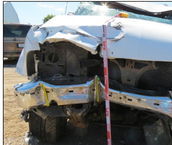
Figure 4. Damage to the front plane of the Chevrolet from the impact with the ET-Plus.
