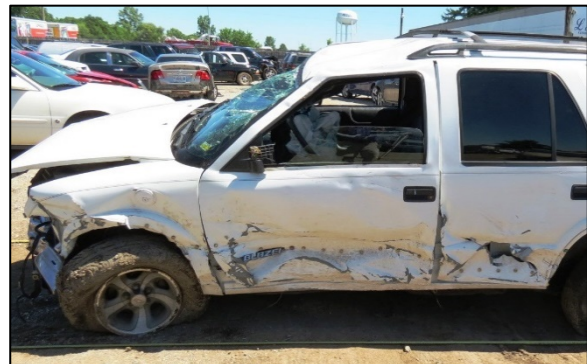
Figure 6. Side view of damage to the Chevrolet’s front bumper and left plane.
