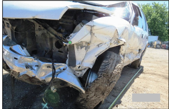
Figure 5. Damage to the left corner of the Chevrolet’s front bumper and left plane from the impact with the damaged guardrail.
