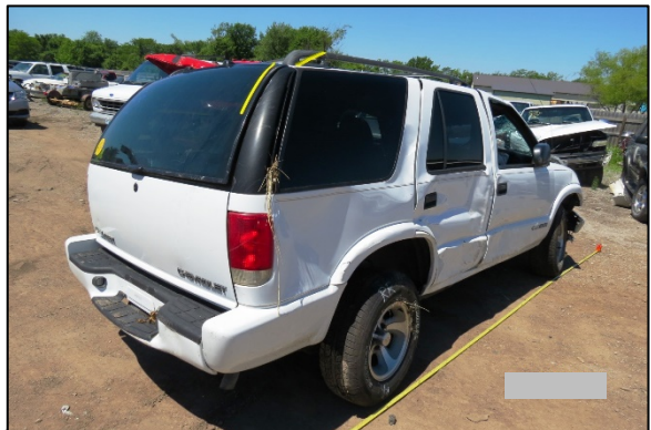
Figure 10. Rollover damage to the right and top planes.
