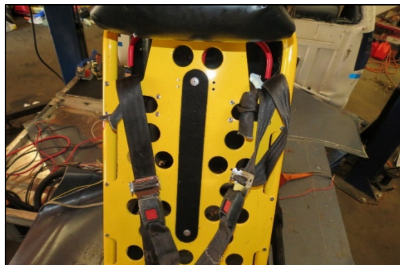
Figure 9. Shoulder/chest restraint straps attached to the backrest.
