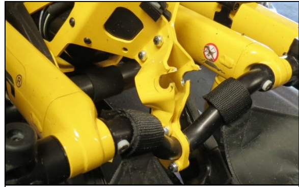
Figure 13. Fractured yoke for the backrest pneumatic lift cylinder pivot pin.
