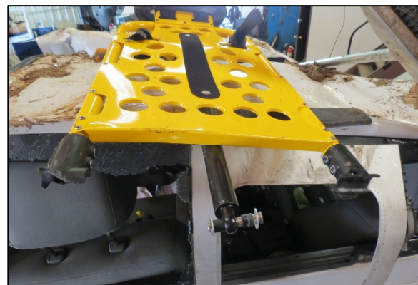
Figure 12. Fractured hinges on the backrest and pneumatic lift cylinder that separated from the yoke.
