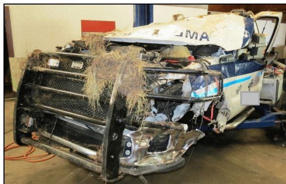
Figure 4. Damage to the left corner of the front bumper from impact with attenuator.
