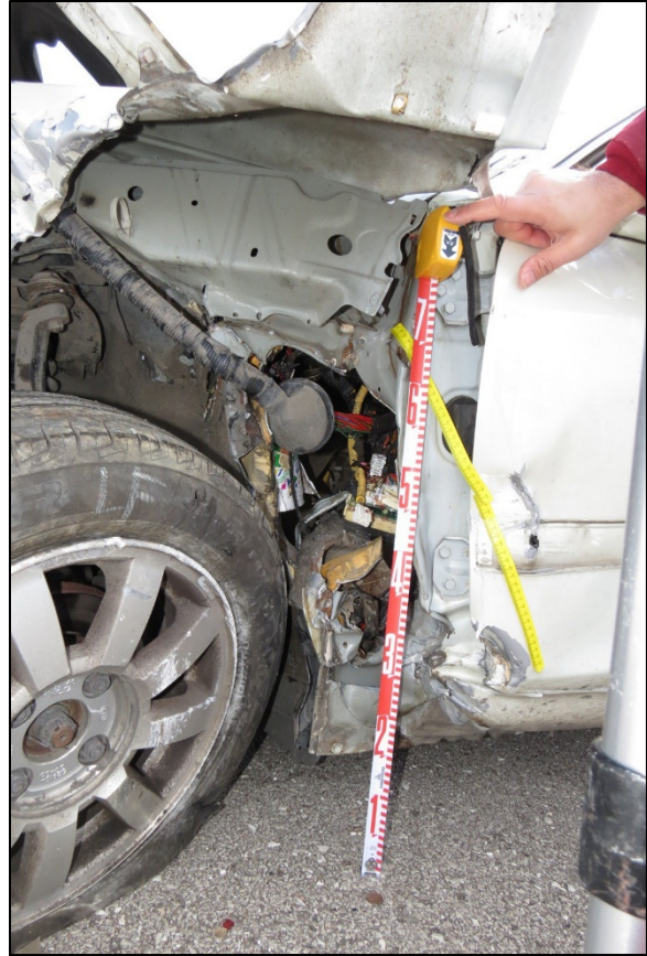
Figure 6. Guardrail penetrated through Kia's left cowl and into the driver's seating position.
