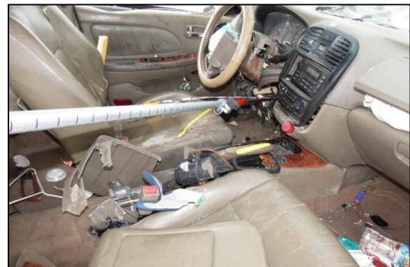
Figure 7. Pole shows path of guardrail penetration through the driver's seating position.
