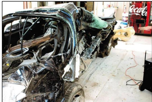
Figure 9. Right-plane deformation to the Pontiac. (Image obtained from the investigating police agency.)
