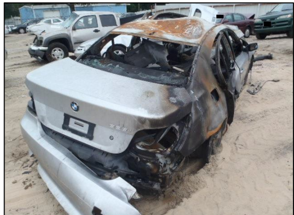
Figure 5. Back-right oblique view of the BMW and the suspected origin of the fire. (Image obtained from an online VIN source.)
