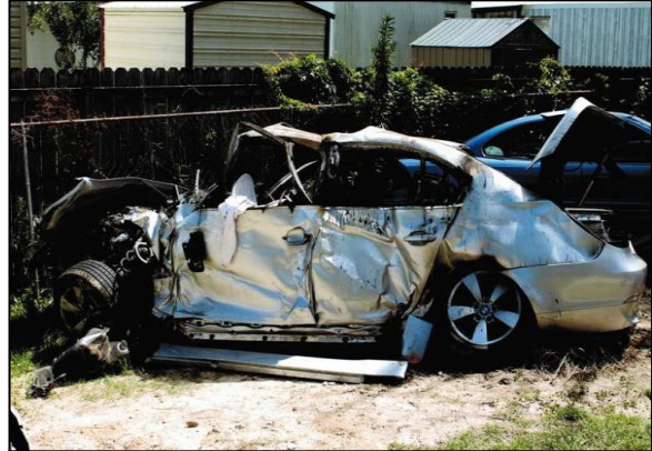
Figure 4. Left plane Event 2 damage to the BMW. (Image obtained from an online VIN source.)
