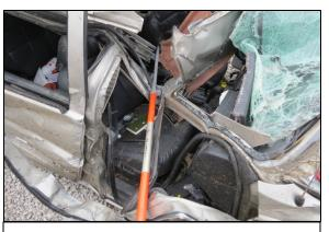
**Figure 9:** Intrusion of right A-pillar/roof side rail/windshield header (Pole represents guard rail).
