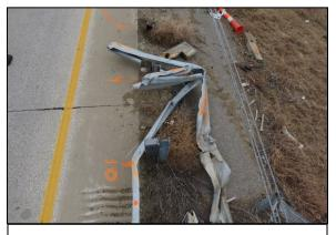
**Figure 4:** Guardrail kinking (west facing lookback view).
