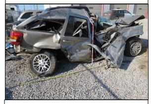
**Figure 8:** Right side rollover damage depicting the maximum vertical deformation located at Row 1.
