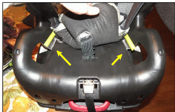
Figure 7. Arrows show the location of tears in plastic on each side of the CRS.
