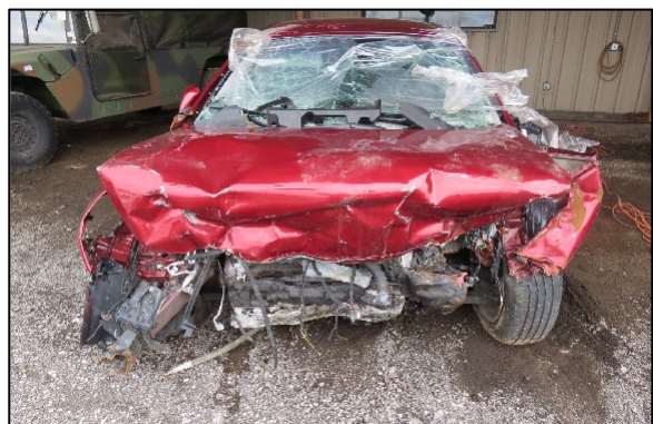
Figure 4. Damage to the front plane of the Hyundai from the impact with the front plane of the Honda.
