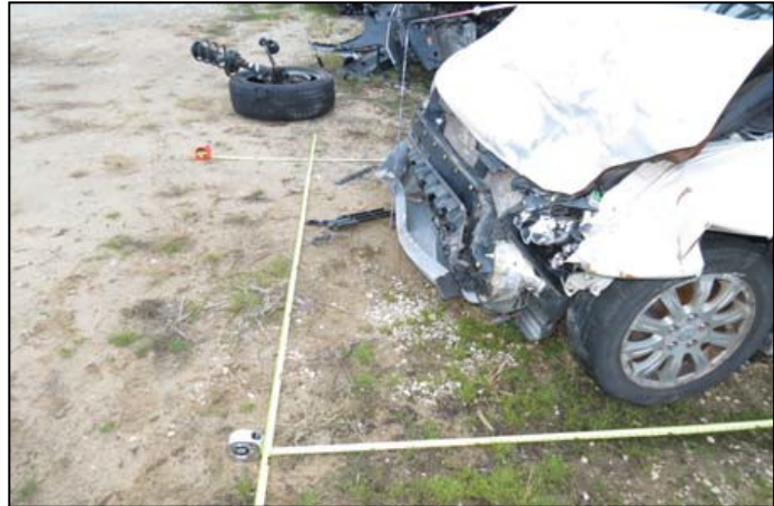
Figure 10. Front end of the damaged Mitsubishi.
