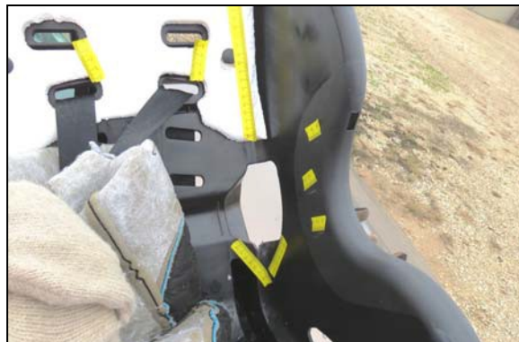
Figure 9. Stress marks/damage to the CRS.
