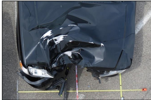
Figure 7: Front crush to the Ford from impact with the utility pole.
