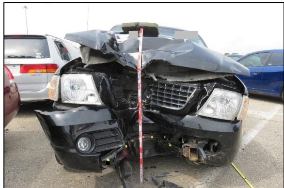
Figure 6: Damage to the Ford's front plane from utility pole impact.
