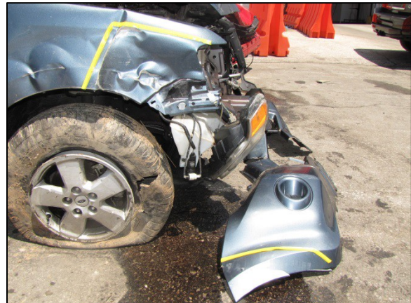
Figure 13. Right side view of the Ford depicting the Event 1 impact damage.
