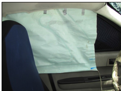
Figure 25. Interior view of the Ford's left IC air bag at the driver's position.
