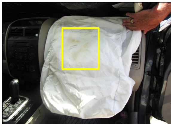
Figure 23. View depicting the make-up transfer to the face of the Ford's passenger frontal air bag.
