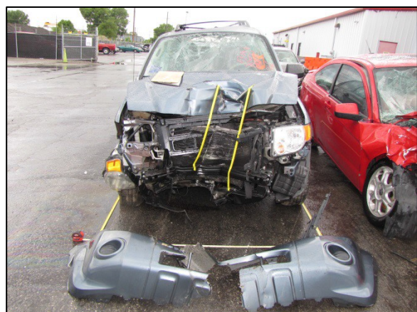
Figure 14. Front view of the Ford depicting the Event 2 impact damage.
