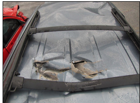
Figure 16. Overhead image of the Ford depicting the roof puncture. Front of the vehicle is toward the top of the image.
