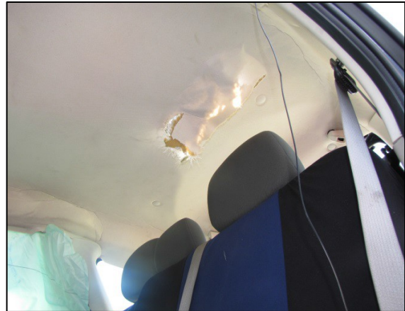
Figure 21. Oblique view of the Ford depicting the roof puncture.
