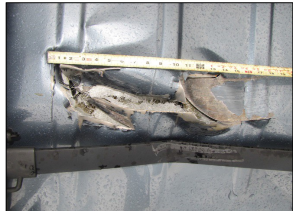
Figure 17. Close-up overhead view of the roof puncture to the Ford with a measuring tape reference.
