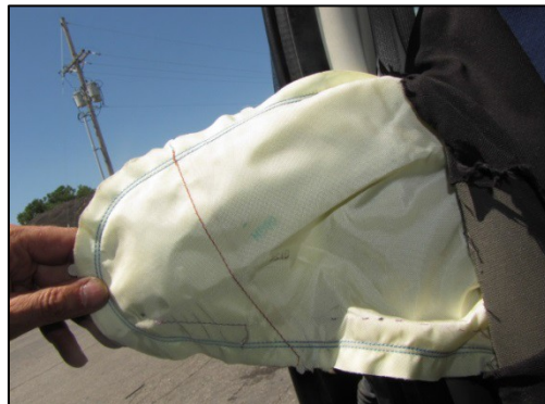
Figure 24. Right-seat-mounted, side-impact air bag of the Ford.
