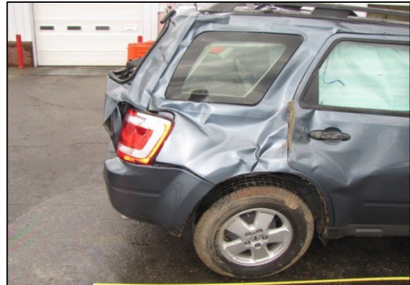
Figure 15. Right-side view of the Ford depicting the rollover damage at the D-pillar.
