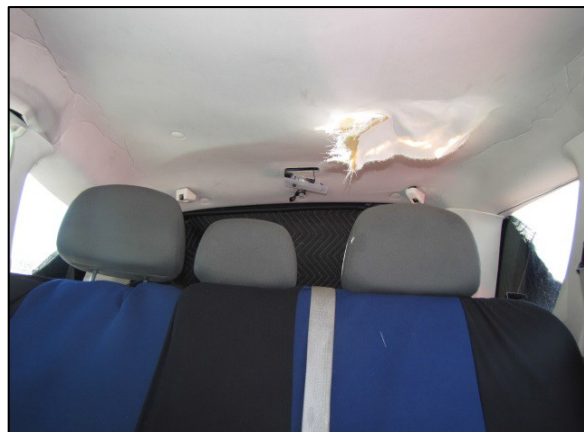
Figure 20. Second-row interior view of the Ford and the puncture to the roof.
