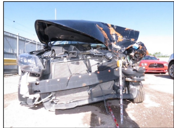
Figure 3. Frontal damage, the 2014 Toyota Avalon.
