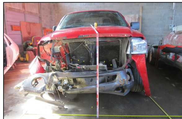
Figure 5. Damage to the Ford's front plane.
