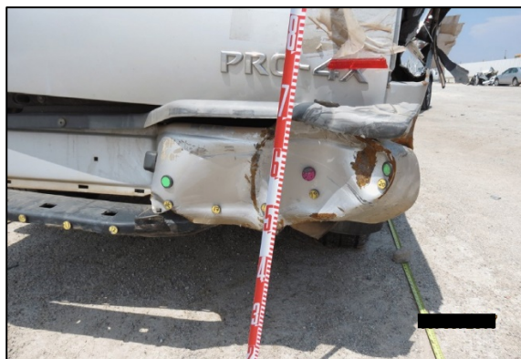
Figure 10. 2010 Nissan Frontier, Rear bumper damage from tree/previous impacts.
