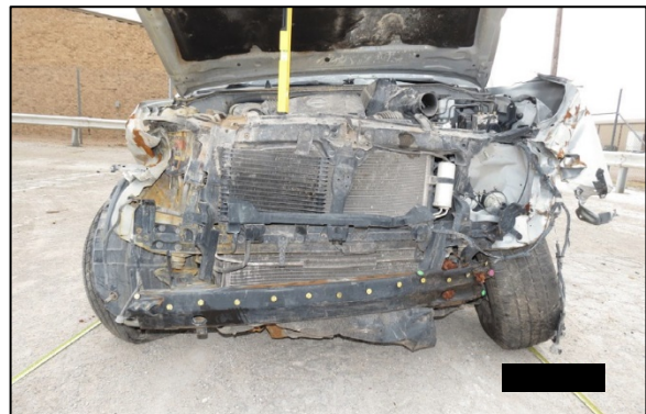
Figure 9. 2010 Nissan Frontier, front plane damage from tree impact.
