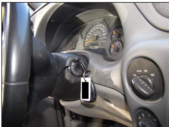
Figure 9: Driver loading and compression of the Chevrolet’s steering column.
