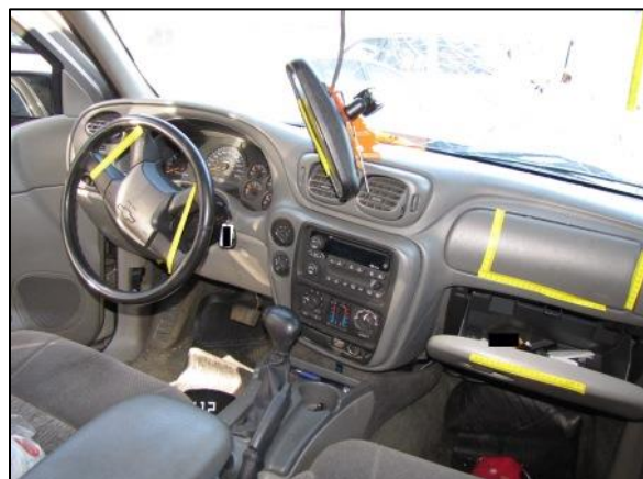
Figure 11: Interior view of the Chevrolet and its non-deployed dual-stage frontal air bags.
