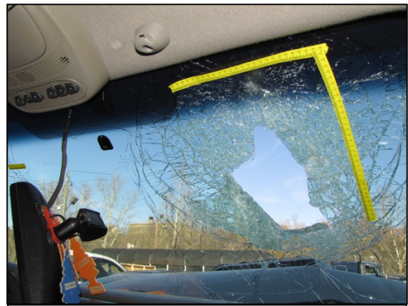
Figure 10: Front row right occupant’s head impacts and holing of the Chevrolet’s laminated windshield.
