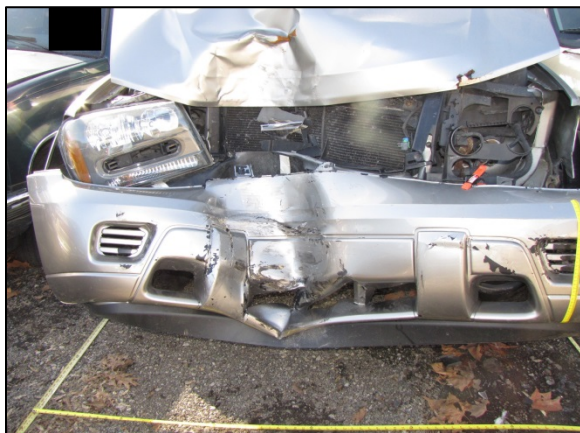
Figure 7: Frontal plane direct contact damage from the utility pole.
