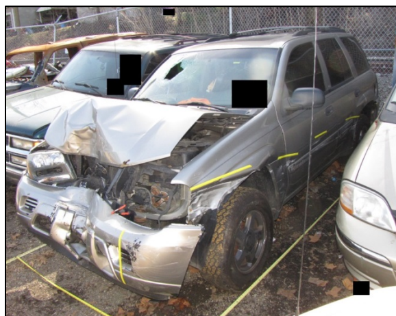
Figure 1: Front left oblique view of the crash-related damage to the 2002 Chevrolet Trailblazer.
