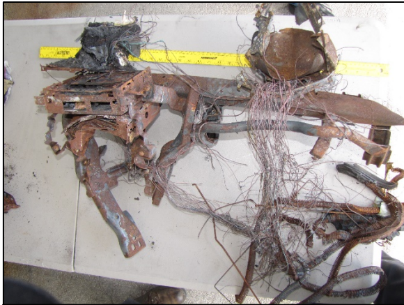
Figure 15. View of the instrument panel section that was cut and removed from the Nissan during the SCI inspection.
