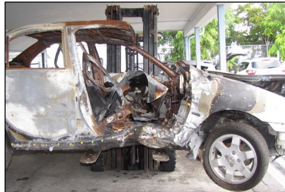
Figure 9. Right view depicting the direct and induced impact damage of the Nissan.
