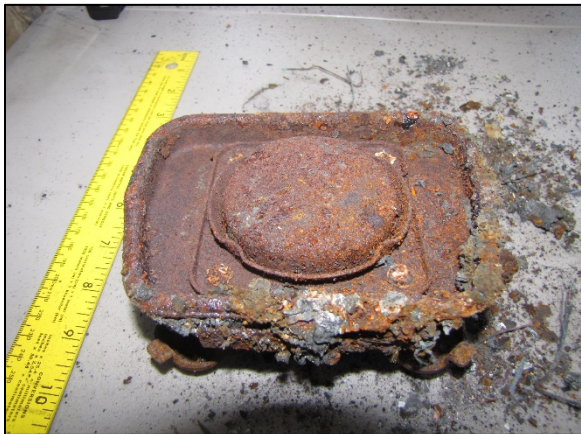
Figure 13. Front side of the Nissan driver's frontal air bag module.
