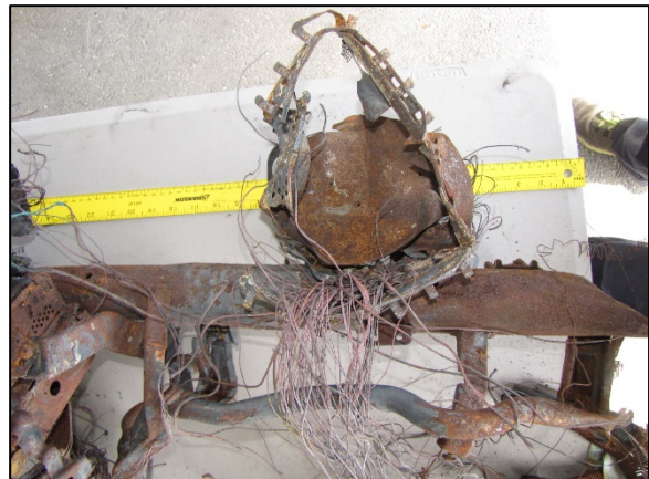
Figure 16. View of the Nissan's ruptured passenger's frontal air bag module which remained attached to the instrument panel.
