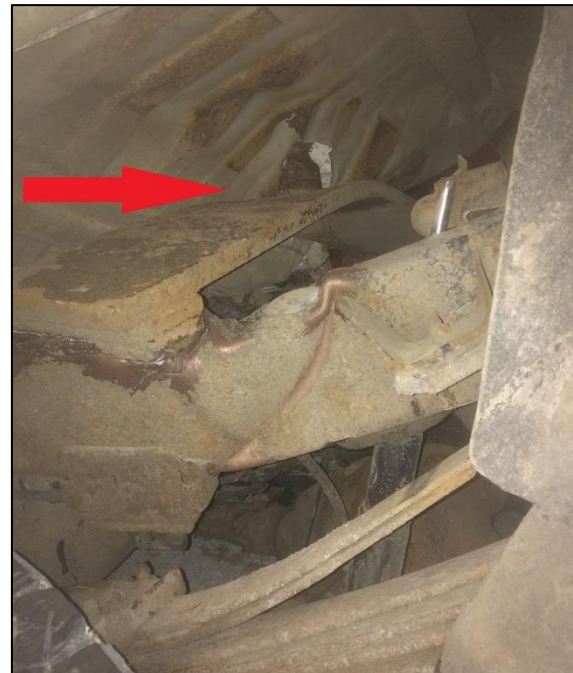
Figure 7. View from left, shows compressed left frame and deformed trailer mount, the 2006 Dodge Ram 3500.
