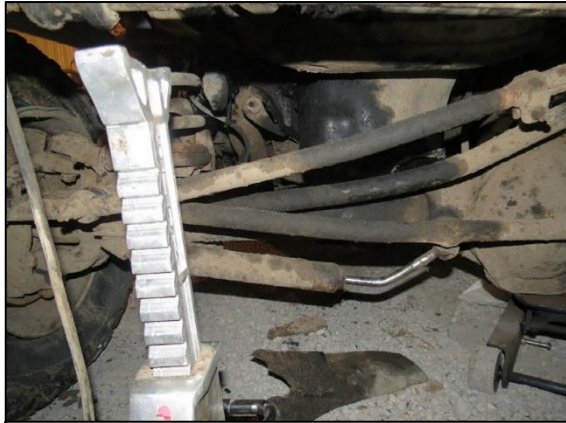
Figure 8. Damaged steering damper, the 2006 Dodge Ram 3500.
