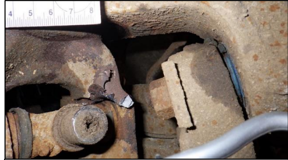
Figure 9. Fractured left axle U-joint, the 2006 Dodge Ram 3500.
