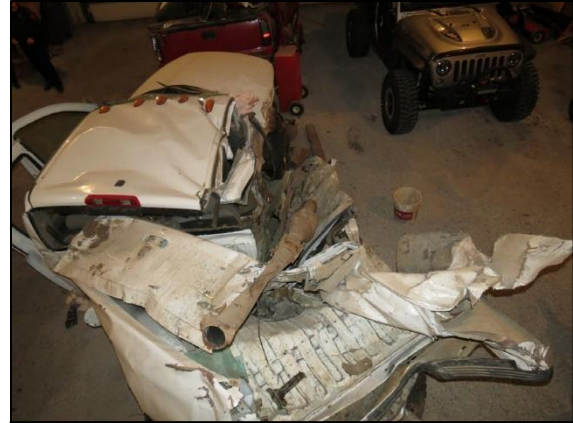
Figure 6. Right plane damage, the 2006 Dodge Ram 3500 pickup.
