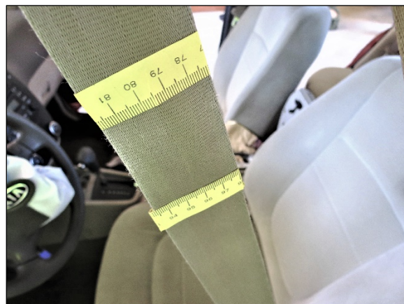
Figure 8. Webbing of the driver seat belt system in the Kia with polymer transfer from the latch plate.
