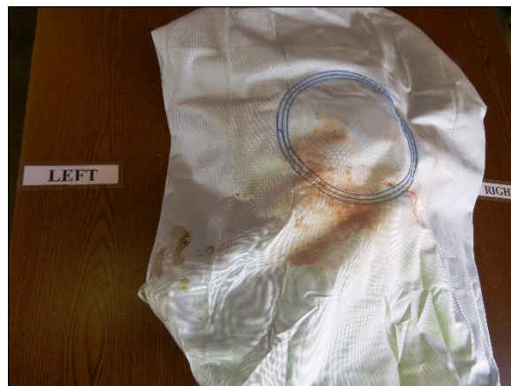
Figure 7. Driver contact evidence on the face of the Kia's deployed driver air bag.
