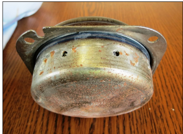
Figure 12. View of the Kia driver's frontal air bag inflator at the time of the SCI vehicle inspection.
