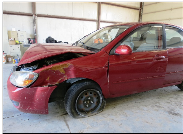
Figure 5. Left view of the Kia and the area of damage to the left front fender from the Ford's left rear wheel.
