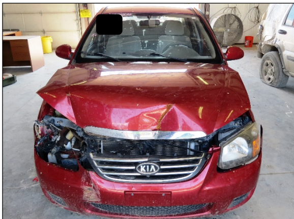
Figure 4. View of the Kia's front plane damage as documented during the SCI inspection.
