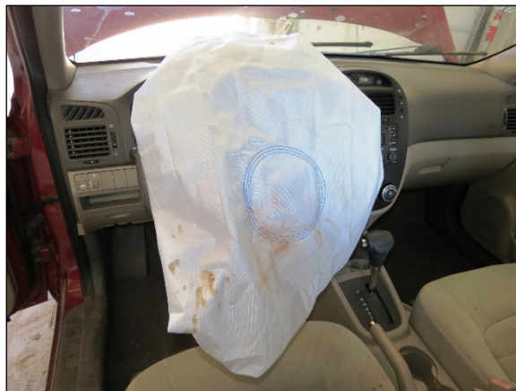
Figure 10. View of the Kia's deployed driver air bag at the time of the SCI vehicle inspection.
