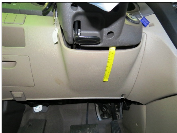
Figure 6. Driver knee contacts to the Kia's left lower instrument panel.
