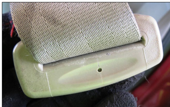
Figure 9. Loading on the Kia driver's latch plate.
