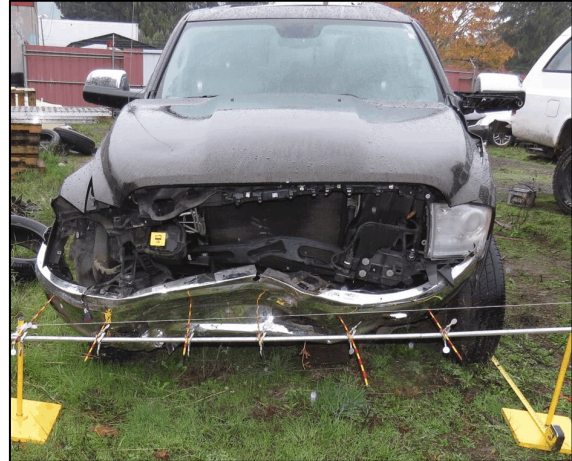
Figure 4. The 2013 Ram 1500, front impact damage.
