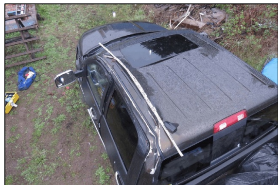
Figure 6. The 2013 Ram 1500, left roof rail damage.
