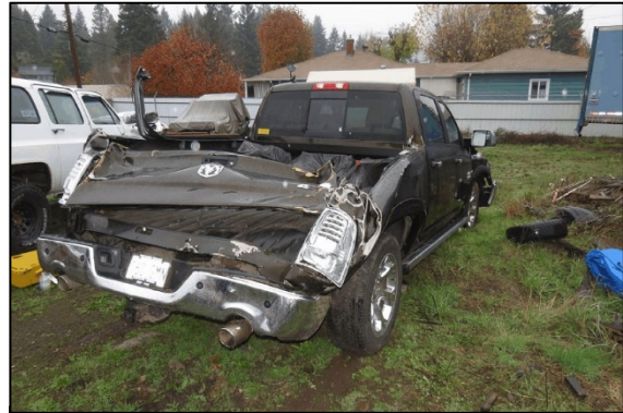
Figure 7. The 2013 Ram 1500, rear plane damage.
