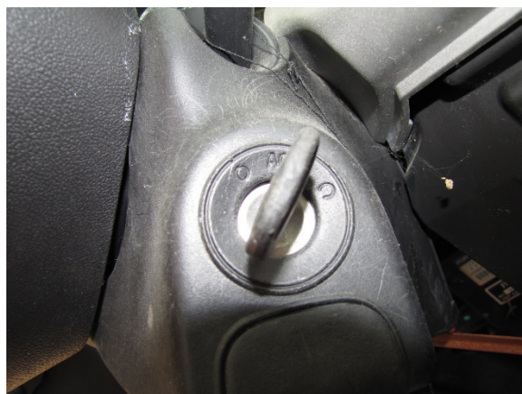
Figure 8. Initial status of the Chevrolet's ignition switch at the SCI vehicle inspection
