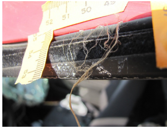
Figure 6. Hair transfer from the driver's head on the outside of the top of the left front window frame, located 30 cm (11.8 in) forward of the driver's head restraint
