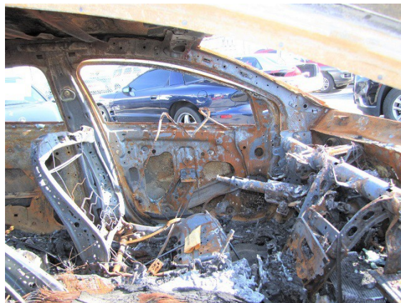
Figure 7. Interior front row damage, 2017 Chevrolet Volt
