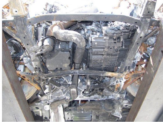
Figure 5. Undercarriage below engine compartment, 2017 Chevrolet Volt
