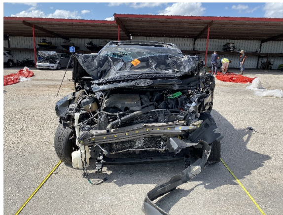
Figure 7. The Ford's front plane damage
