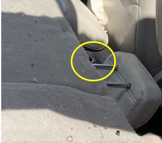
Figure 13. Top tether load mark at top second-row, center seat back
