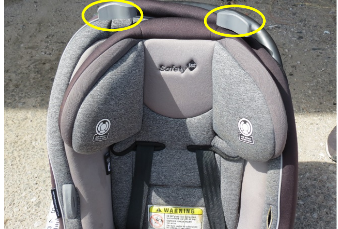
Figure 14. CRS headrest and shoulder strap adjustment levers
