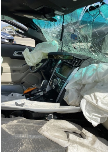
Figure 10. The Ford's deployed frontal air bags
