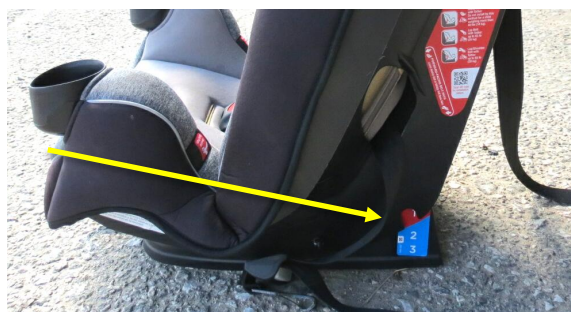
Figure 12. Left side of CRS with incline adjustment at the "1" (most upright) position
