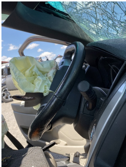
Figure 8. The Ford's steering wheel/column deformation
