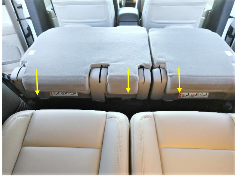
Figure 6. Second-row top tether anchor points
