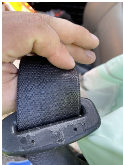
Figure 9. Frictional abrasions on the driver's latch plate
