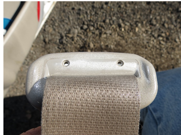
Figure 19. Loading evidence on the latch plate of the Kia's front-row right occupant seat belt system
