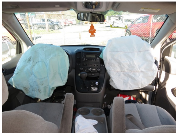
Figure 20. Deployed frontal air bags in the Kia
