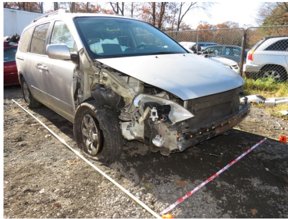
Figure 1. Front right oblique view of the guardrail damage to the Kia Sedona
