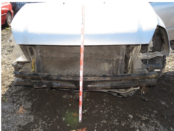
Figure 16. Exposed bumper beam of the Kia
