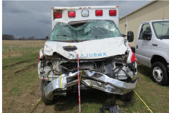
Figure 6. Front plane damage
