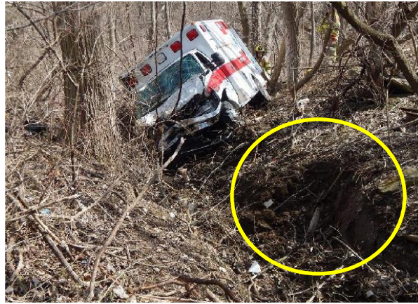
Figure 5. Police photo showing impact of upper/right-front corner of the patient compartment into ditch bank and the ambulance at final rest
