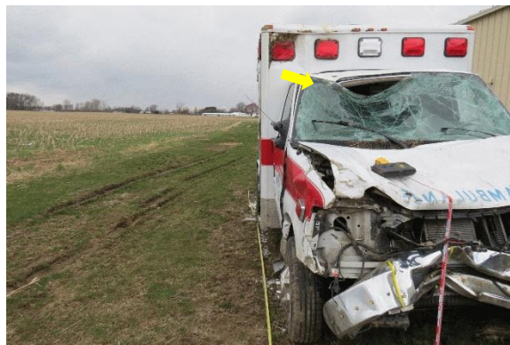
Figure 7. Maximum vertical crush occurred at the right windshield header
