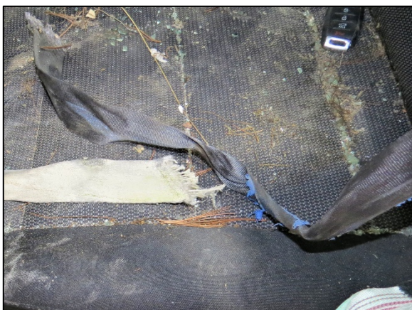
Figure 9. Webbing of the driver seat belt system in the Kia with blue fabric transfer from the driver's clothing.
