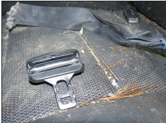
Figure 11. Latch plate of the Kia's driver seat belt system with the lightweight locking portion missing.
