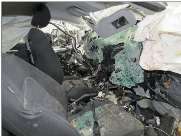
Figure 7. Left-facing view of the Kia's front row and the visible longitudinal intrusion of the instrument panel.
