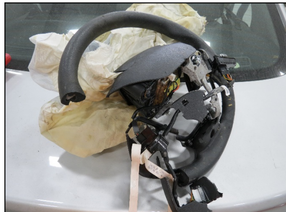
Figure 8. Sheared steering wheel and fractured assembly resultant from loading by the Kia's driver.
