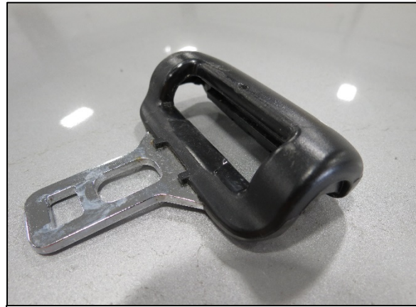
Figure 12. Latch plate of the front passenger's seat belt system with the lightweight locking portion missing.
