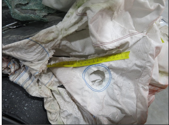
Figure 16. Large tear on the left side of the Kia's passenger's frontal air bag.
