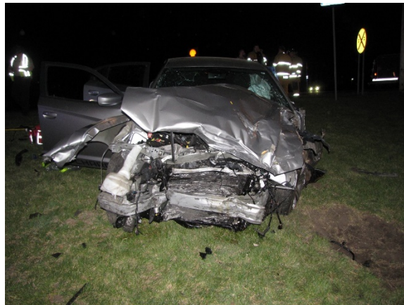
Figure 7. The 2014 Dodge Charger, front plane damage (police photo)
