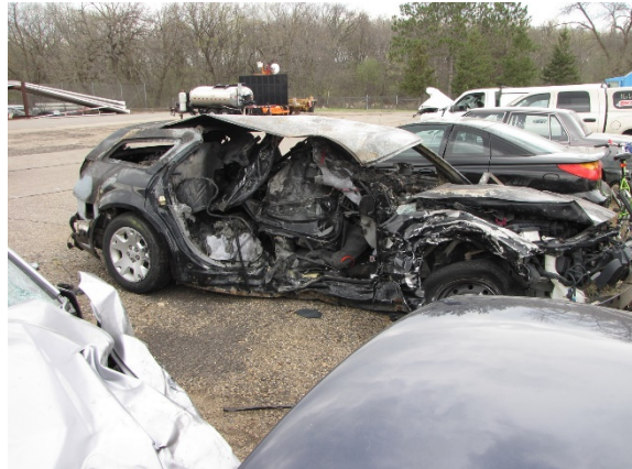
Figure 6. The 2007 Dodge Magnum, right plane damage (police photo)
