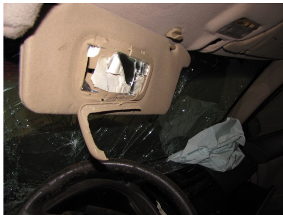
Figure 14. Interior view depicting the left sun visor and fractured vanity mirror of the Honda
