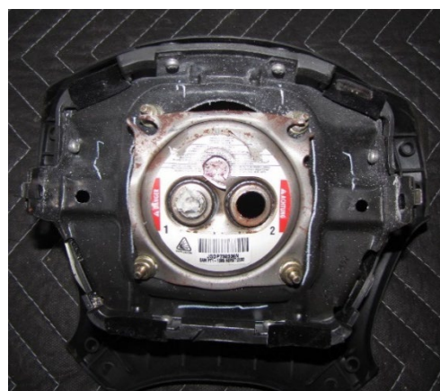
Figure 22. Image depicting the backside of the Honda driver's frontal air bag module
