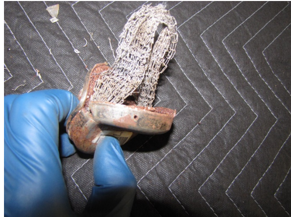
Figure 24. Side view depicting the Honda's ruptured and separated driver's frontal air bag inflator cap
