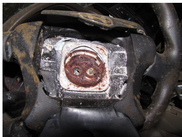
Figure 18. Image of the Honda's driver's frontal air bag module depicting the condition of the ruptured inflator. Image taken five months post-crash
