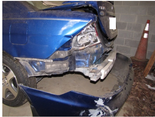
Figure 10. Close-up view of the secondary impact damage to the Honda's quarter panel
