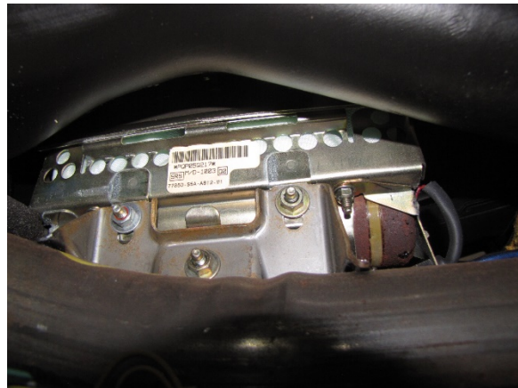
Figure 26. View of the Honda's passenger air bag module and its identification label
