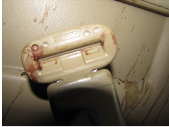
Figure 16. Image depicting the latch plate of the Honda driver's seat belt in the buckle receiver
