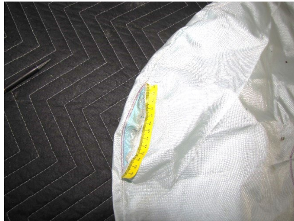
Figure 20. Image depicting the tear in the peripheral seam of the Honda's driver's frontal air bag
