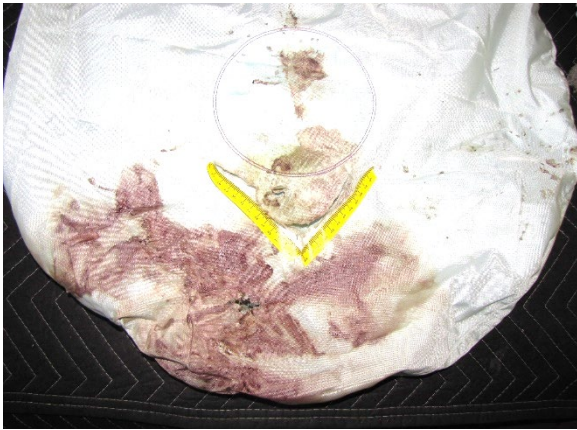
Figure 19. Image depicting the tear in the fabric at the center of the Honda's driver's frontal air bag
