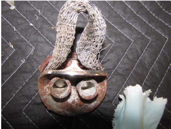
Figure 23. Back view depicting the Honda's ruptured and separated driver's frontal air bag inflator cap
