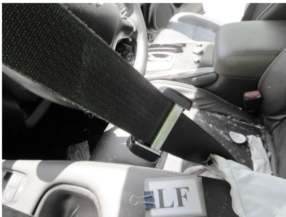
Figure 14. Latch plate loading evidence on the webbing of the Infiniti driver's seat belt system
