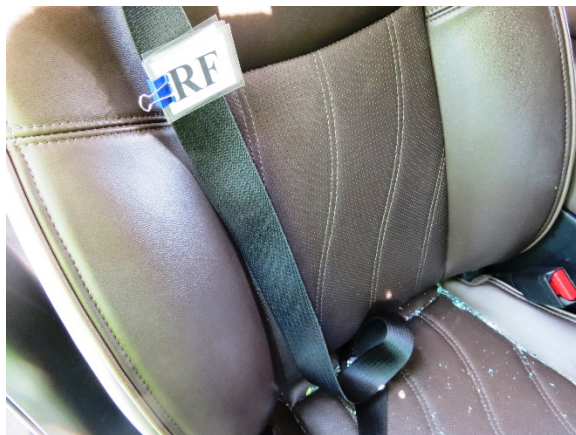
Figure 15. Loading evidence to the front right passenger's seat belt system in the Infiniti
