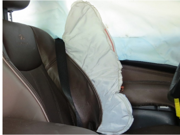
Figure 18. Left-facing view of the driver's deployed seat-mounted air bag in the Infiniti
