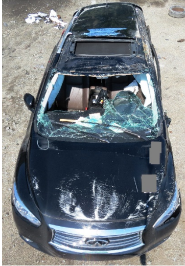
Figure 9. View of the Infiniti's rollover damage
