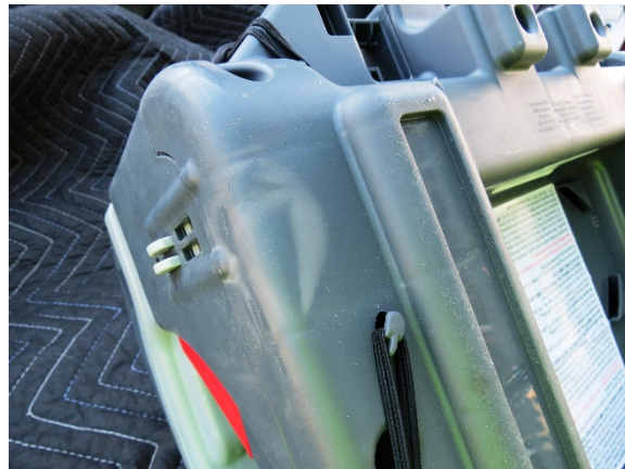
Figure 23. Loading stress marks on the lower left corner of the CRS base
