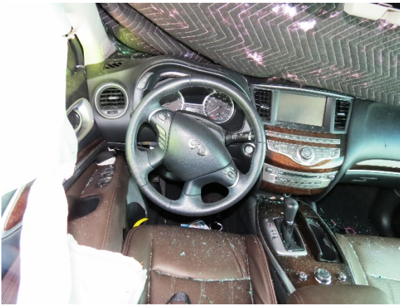
Figure 10. Intrusion of the left front door of the Infiniti that resulted in lateral deformation to the driver's seat
