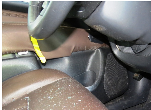
Figure 13. Driver contact to the left front door panel and underside of the steering column in the Infiniti
