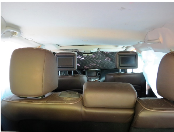
Figure 12. Deformation to the greenhouse structure of the Infiniti as viewed forward-facing from the third row
