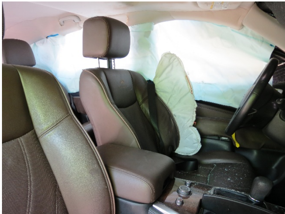
Figure 19. View of the deployed left IC air bag for the driver and second row positions in the Infiniti
