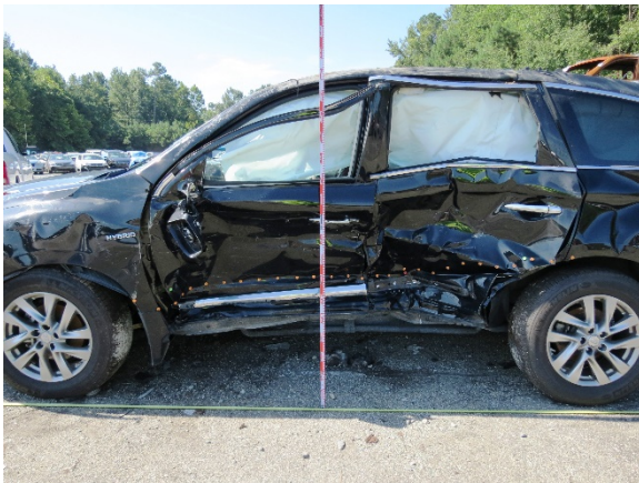
Figure 7. Left plane damage to the Infiniti as observed at the time of the SCI vehicle inspection
