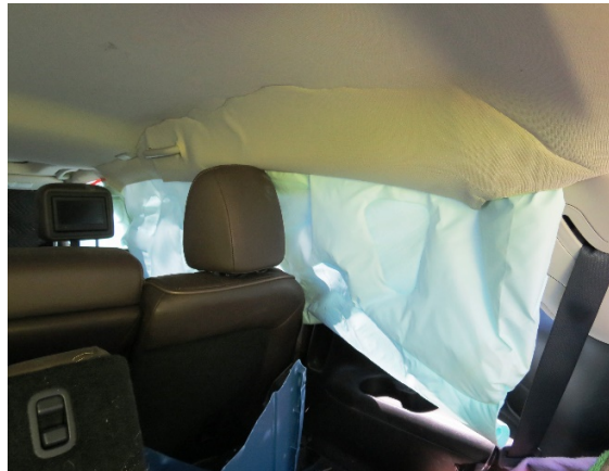
Figure 20. Forward-facing view of the deployed right IC air bag in the Infiniti from the third row
