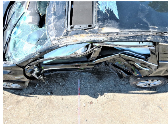
Figure 8. Overhead perspective of the SCI documentation of the Infiniti's left plane damage
