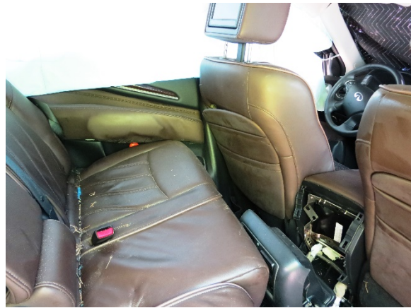
Figure 11. Left rear door and left B-pillar intrusion in the Infiniti that resulted in deformation to the second row left seat cushion, driver's seat, and center console
