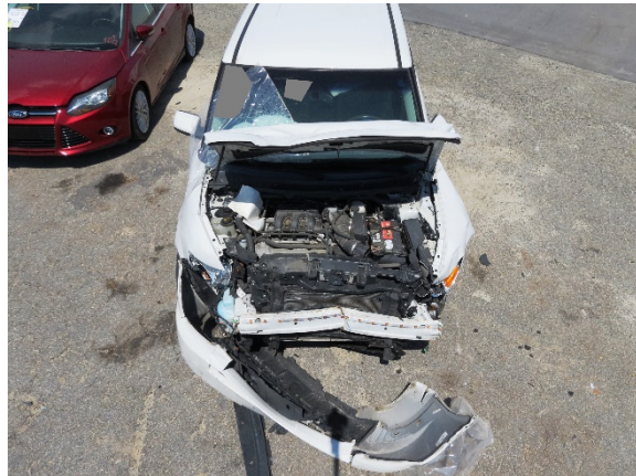
Figure 26. Overhead view of the damage profile to the Ford's front plane
