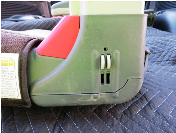
Figure 22. View of the left aspect of the CRS and stress marks to the shell
