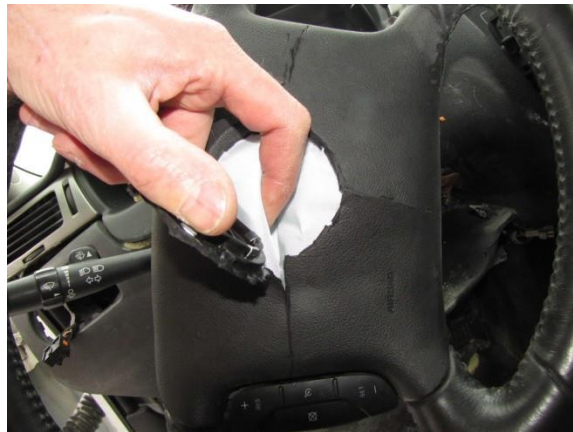
Figure 13. Image depicting the presence of the undeployed air bag housed in the driver's frontal air bag module in the Chevrolet
