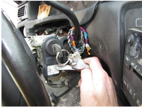
Figure 19. Image depicting the ignition switch of the Chevrolet in the “Accessory” position with a force application applied at the attached items
