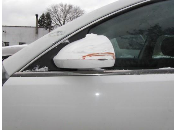
Figure 9. Image depicting the swiping abrasion/paint transfer to the left mirror of the Chevrolet (Event 2)
