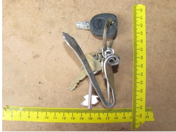
Figure 16. Image depicting the Chevrolet's broken ignition key, 32 mm key ring, and additional attached items
