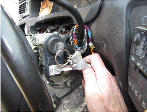
Figure 18. Image depicting the ignition switch of the Chevrolet in the “Run” position
