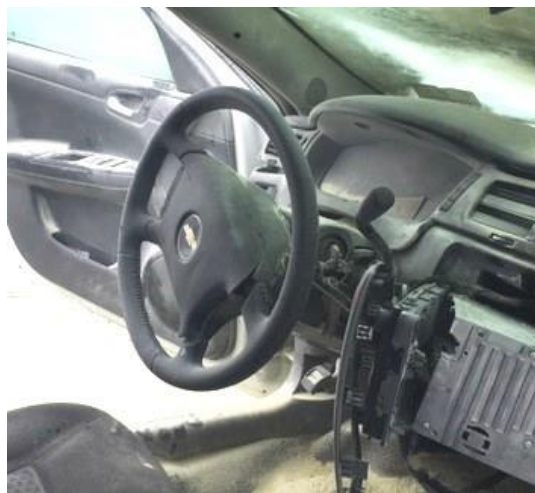
Figure 17. On-scene police image of the steering wheel and column depicting the position of the ignition switch
