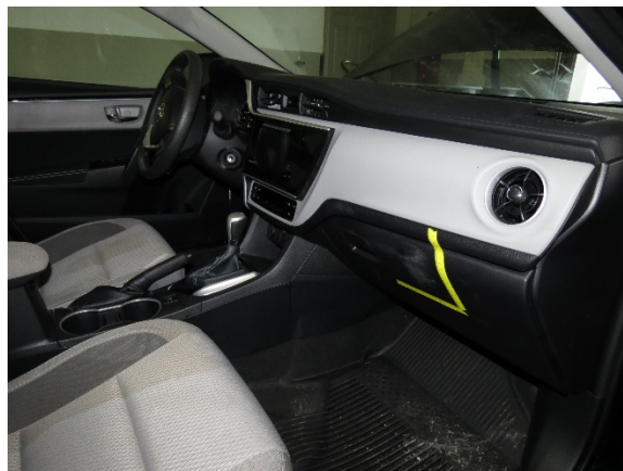
Figure 7. Probable front-row right occupant knee contact to the right lower instrument panel
