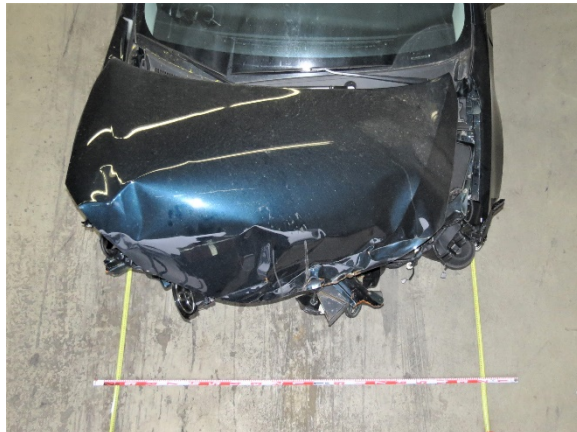
Figure 6. Overhead view of the Corolla's damage profile
