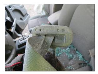
*Figure 12. Webbing gathered in the Nissan driver's latch plate as a result of occupant loading during the crash*
