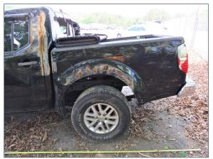
Figure 9. Rollover damage to the rear aspect of the Nissan's left plane
