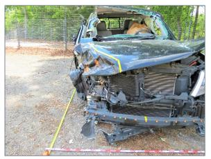
Figure 6. Front view of the Nissan and the Event 1 impact damage to the right front corner
