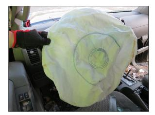
Figure 13. View of the deployed driver's frontal air bag in the Nissan at the time of the SCI vehicle inspection
