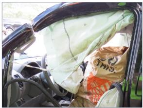
Figure 14. View of the left IC air bag captured at the top of the B-pillar as observed by the SCI Investigator
