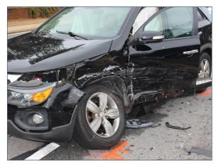
Figure 26. Left front oblique view of the damage pattern to the Kia (on-scene law enforcement image)
