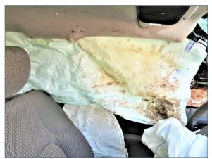
Figure 15. Interior aspect of the deployed left IC air bag. Note the clean folds and contact void at the B-pillar area
