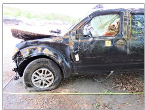
Figure 8. Left view of the Nissan and the Event 4 rollover damage to the forward aspect
