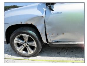
Figure 24. Secondary damage to the left plane of the Toyota from the sideswipe by the Chevrolet
