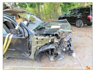
Figure 7. Right view of the front right corner damage to the Nissan from the impact with the Chevrolet
