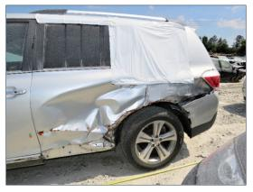
Figure 23. Direct contact damage to the rear aspect of the Toyota's left plane
