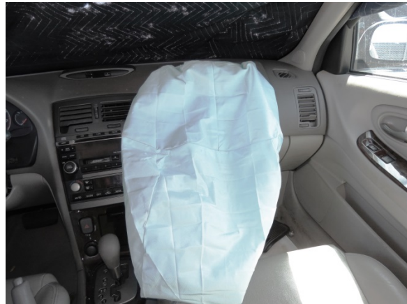
Figure 16. Deployed passenger's frontal air bag in the Nissan
