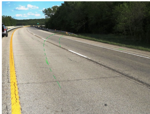
Figure 3. East-facing view of the Nissan's CW yawing tire marks on approach to impact with the guardrail
