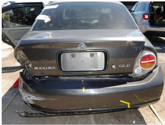
Figure 12. View of the Nissan's rear-plane damage
