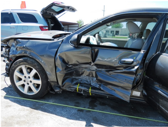
Figure 11. Left view depicting the damage at the left-front door of the Nissan
