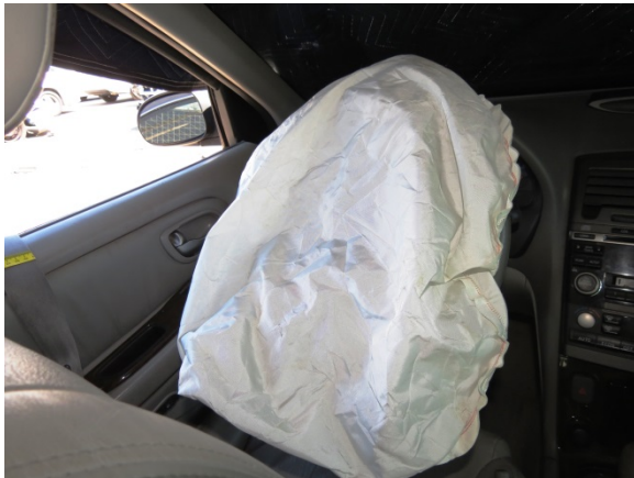
Figure 15. View of the deployed driver's frontal air bag in the Nissan
