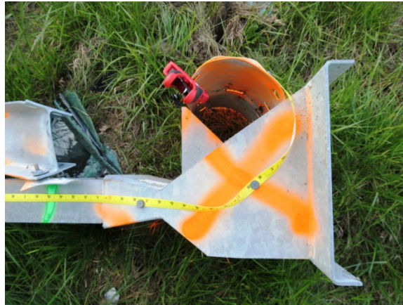
Figure 5. West-facing view of the ET-Plus end terminal impact head and deformed W-beam guardrail in their displaced position following the crash
