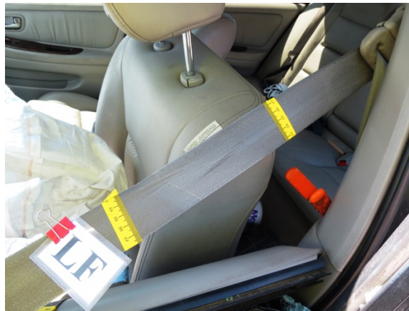
Figure 14. Area of D-ring loading to the Nissan driver's lap and shoulder seat belt system
