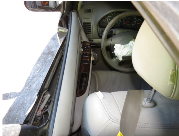
Figure 13. Overhead view of the intruded left front door engaged against the driver's seat of the Nissan
