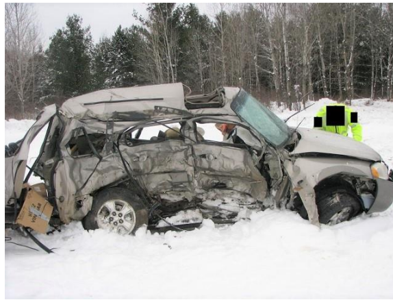
Figure 7. Right plane damage, the 2001 Mazda Tribute (police photo)
