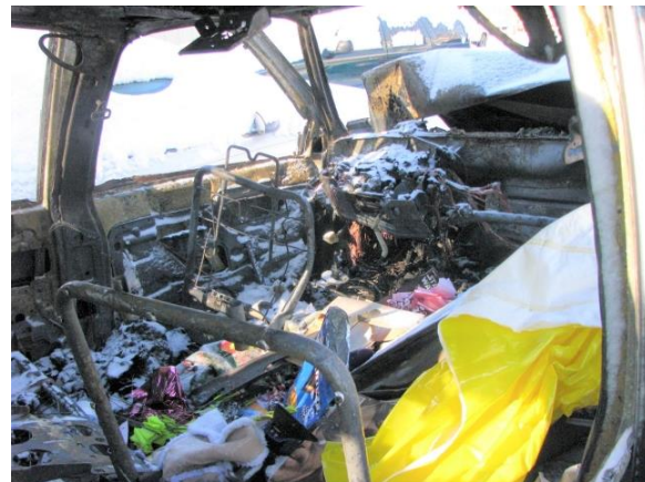
Figure 5. Interior fire damage, the 1995 GMC Suburban (police photo)
