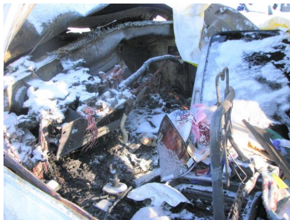
Figure 6. Front row showing longitudinal intrusion, the 1995 GMC Suburban (police photo)
