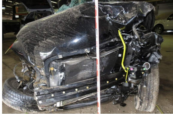
Figure 5. Damage to front plane from impact with ET-Plus
