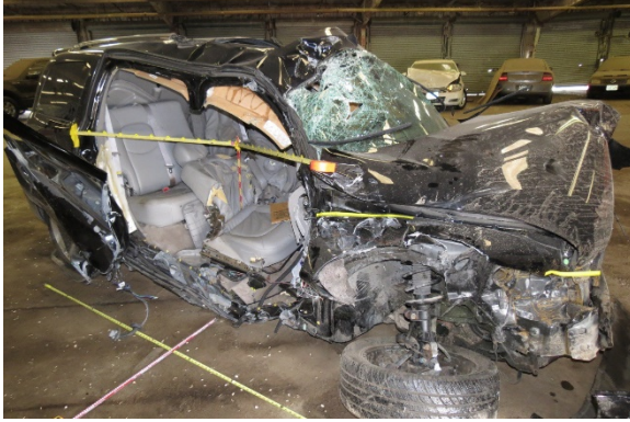
Figure 7. Damage to the right plane of the Chevrolet from impact with the deformed guardrail
