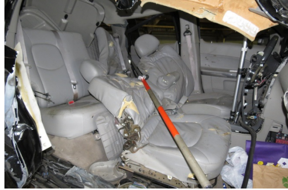
Figure 8. Pole shows path of guardrail penetration into Chevrolet's occupant compartment
