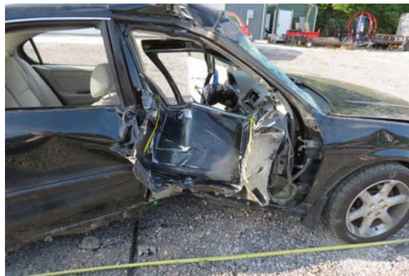
Figure 8. Right plane damage from the guardrail head impact (door sheet metal placed on by researcher)
