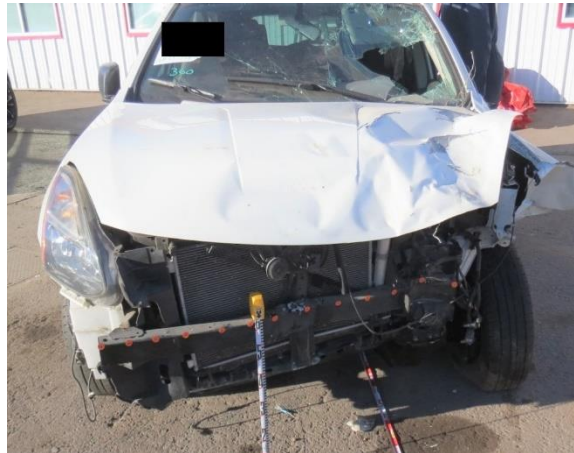
Figure 4. The 2015 Nissan Rogue, front plane damage
