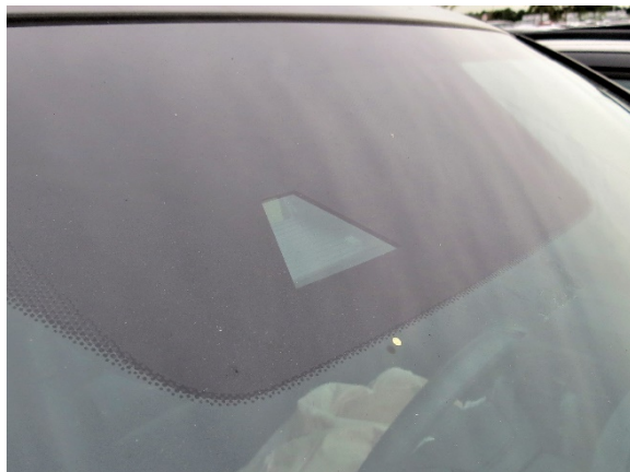
Figure 11. View of the Honda's optical sensor for the FCW and LDW systems
