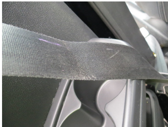
Figure 7. Latch plate loading evidence on the driver's seat belt system in the Honda
