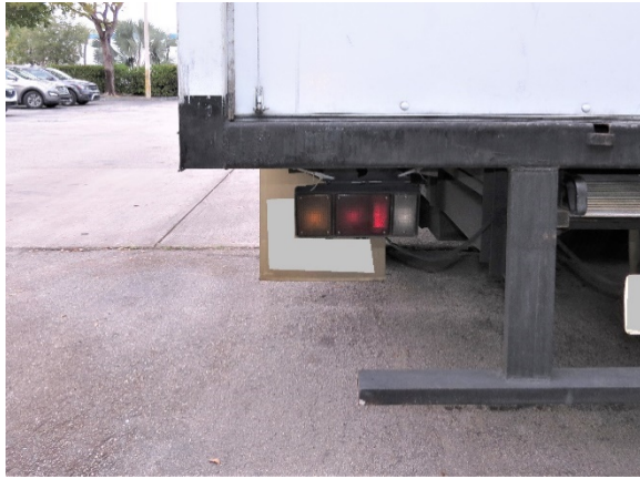
Figure 14. Area of impact to the rear plane of the Isuzu
