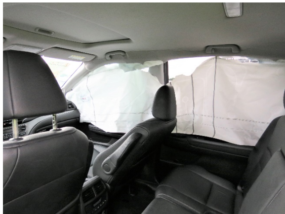
Figure 9. View from the second row of the deployed right IC air bag in the Honda
