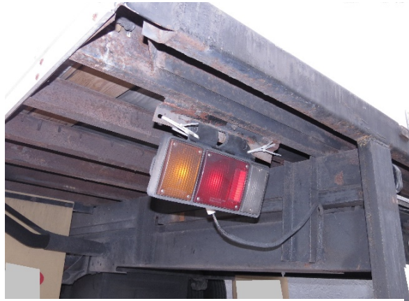
Figure 15. Damaged left rear taillight of the Isuzu
