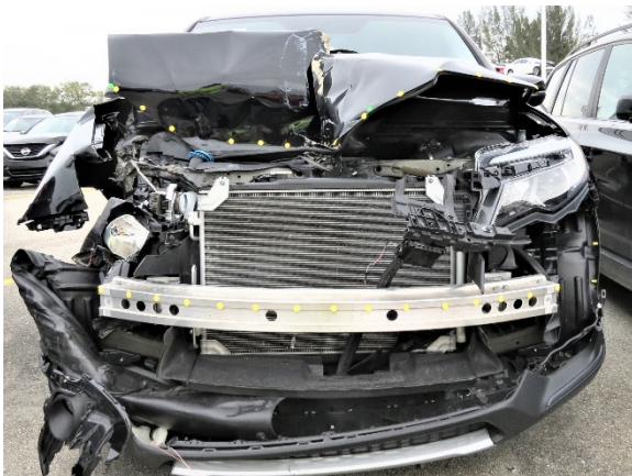
Figure 4. Front plane damage to the Honda as documented during the SCI vehicle inspection
