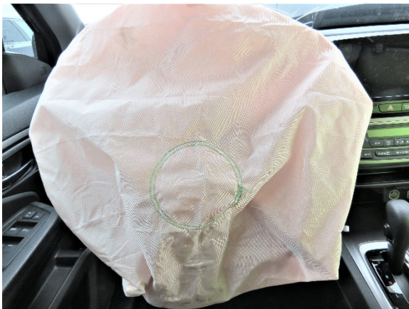
Figure 8. View of the deployed driver's frontal air bag in the Honda at the time of the SCI inspection
