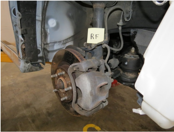
Figure 6. Right front brake assembly of the Toyota
