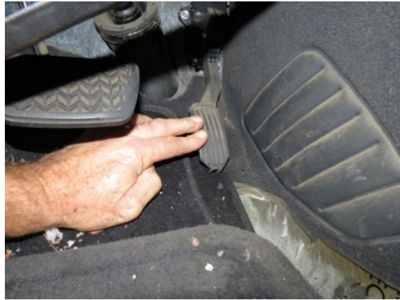
Figure 7. Recall-modified Denso accelerator pedal fully depressed against the carpeted floor mat
