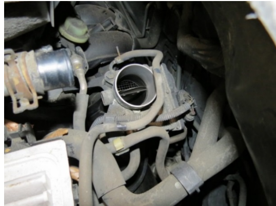
Figure 9. Throttle plate of the Toyota fully open during the check-out
