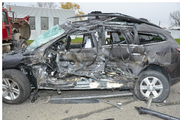
Figure 7. On-scene view of the left plane impact damage to the 2014 Chevrolet Traverse, prior to the removal of the left front door (image provided by the investigating law enforcement agency)
