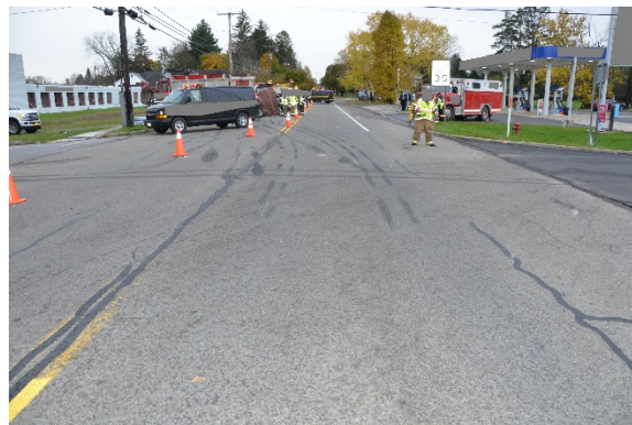
Figure 4. South-facing on-scene image depicting the vehicles' post-impact tire marks (on-scene law enforcement image)
