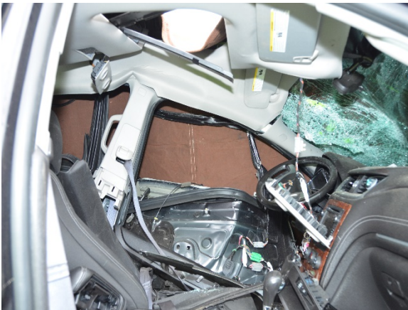
Figure 10. Left-facing view of the intruded driver’s door prior to its removal (image provided by the investigating law enforcement agency)
