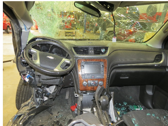
Figure 11. Forward-facing view of the deformed steering wheel and left A-pillar/left instrument panel deformation at the time of the SCI inspection
