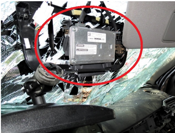
Figure 7. Front sensor camera mounted to top center windshield, the 2018 Honda Accord
