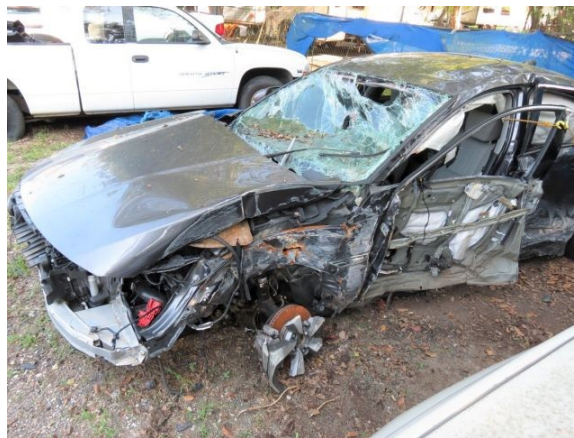
Figure 6. Left plane damage, the 2018 Honda Accord
