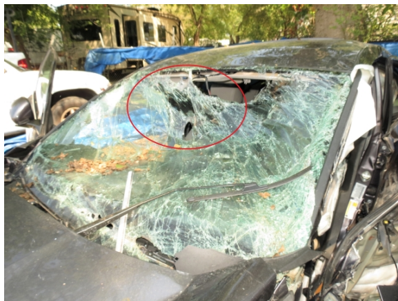
Figure 8. Front sensor camera mounted to top center windshield, the 2018 Honda Accord
