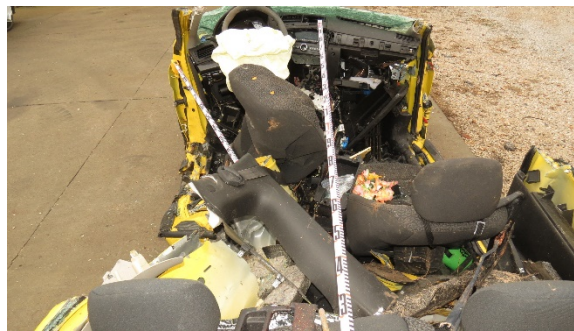
Figure 8. Intrusion into the Pontiac driver's seating area and displacement of the driver's seat
