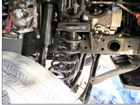
Figure 18. Left-facing view of the right front suspension showing rearward deflection of the spring and shock
