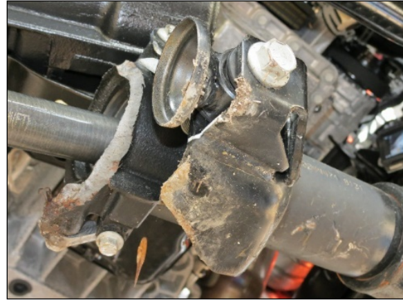
Figure 21. Underside view of the direct contact damage to the fractured front axle and steering damper mount
