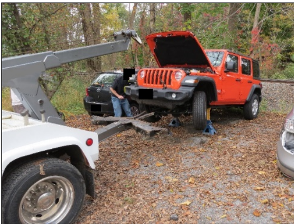
Figure 12. Elevation of the Jeep using a recovery vehicle and jack stands during the SCI vehicle inspection
