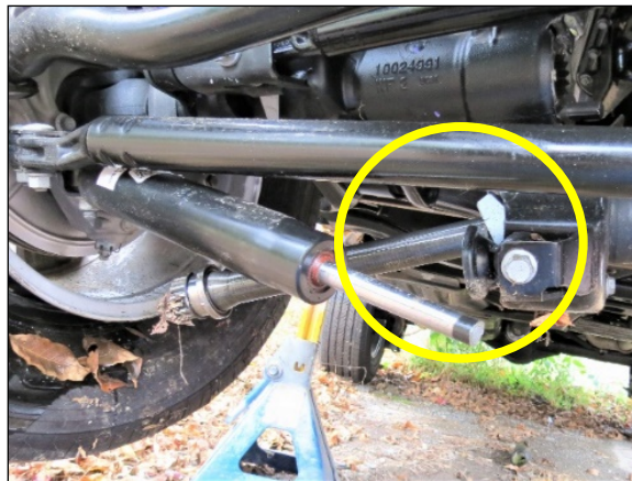
Figure 16. View of the Jeep's sheared steering damper at the right front axle position
