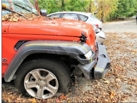
Figure 8. Right plane view of the front of the Jeep and the crash damage
