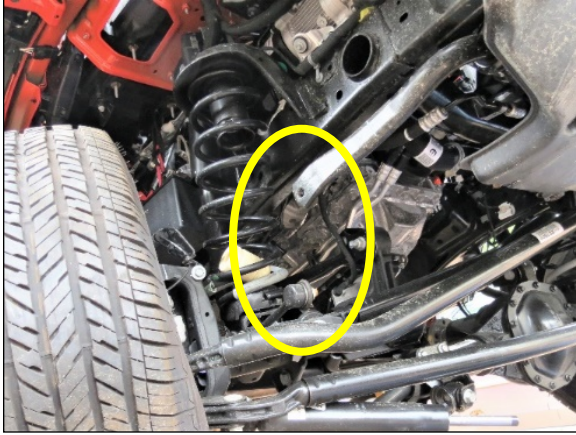
Figure 17. View of the Jeep's separated front sway bar linkage
