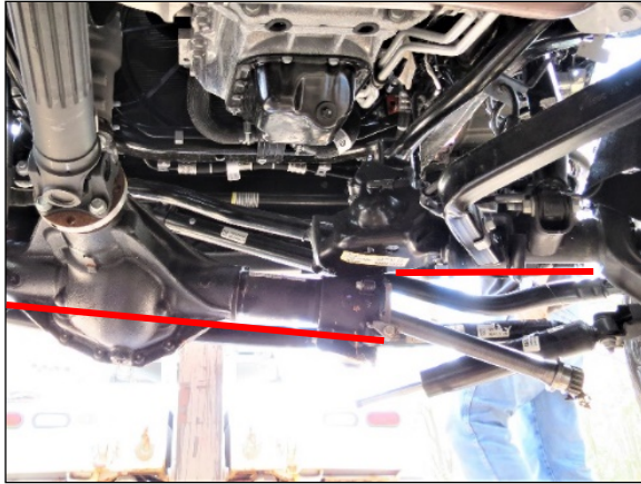
Figure 20. Forward-facing view of the Jeep's fractured front axle assembly
