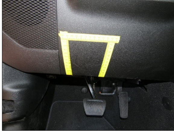
Figure 9. Driver left knee contact to the Jeep's left lower instrument panel
