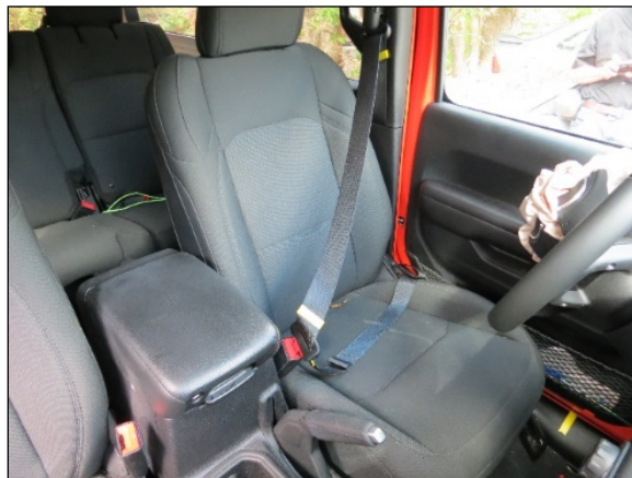
Figure 10. Driver's seat belt system in the Jeep, with areas of loading evidence highlighted by yellow tape
