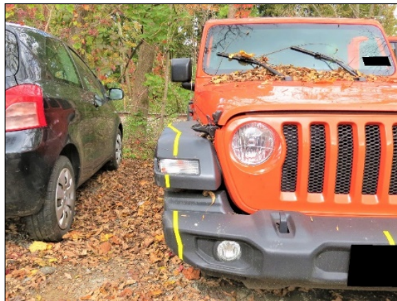
Figure 7. View of the damage to the Jeep's right front corner, from a frontal perspective
