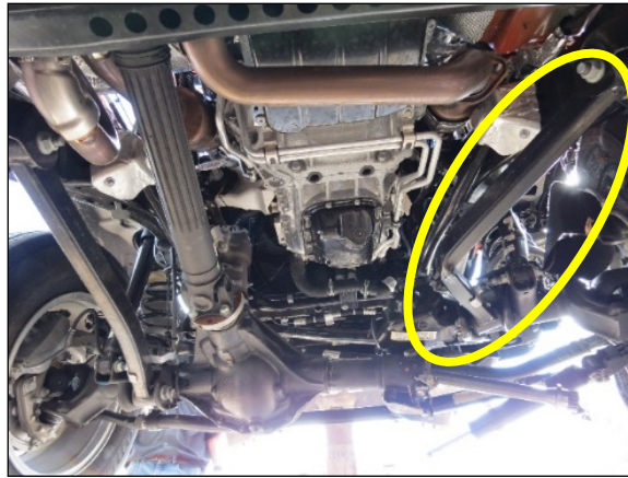
Figure 19. Forward-facing view of the Jeep's bent right control arm and undamaged left control arm
