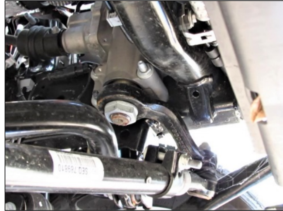
Figure 15. Center link, pitman arm, and steering gear of the Jeep's steering system
