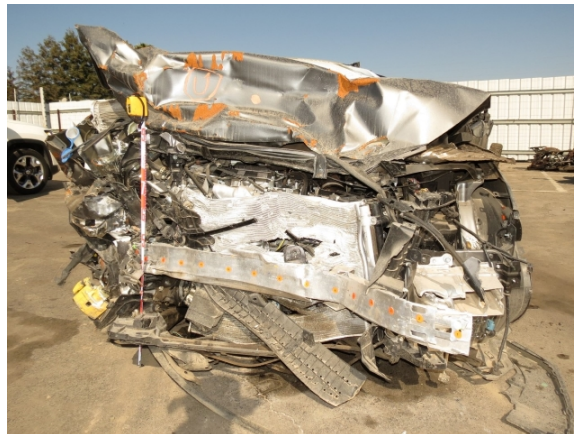
Figure 4. Front plane damage, 2019 Honda Civic
