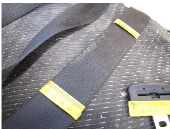
Figure 5. Driver's seat belt components, driver loading evidence, the 2014 Dodge Journey
