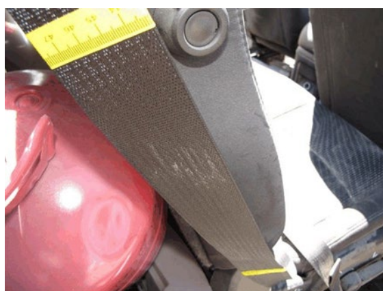
Figure 6. Second row right position seat belt webbing, occupant loading evidence, the 2014 Dodge Journey
