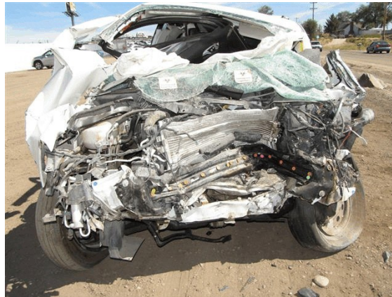
Figure 4. Front plane crush damage, the 2014 Dodge Journey
